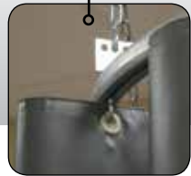
Curved roller track with chain support
